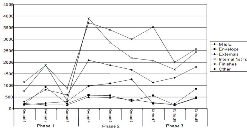
Further analysis of the data in figure one and figure two illustrate both the external works and the main structural envelope delivered a constant level of quality across all nine projects.
