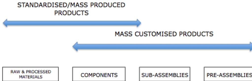
Figure 1: Ranges of Standardised and Customised products combined with levels of preassembly
