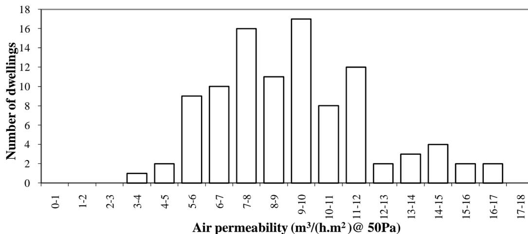
Figure 1: Mean air permeability of dwellings built to Part L1 2002. After Grigg (2004)
