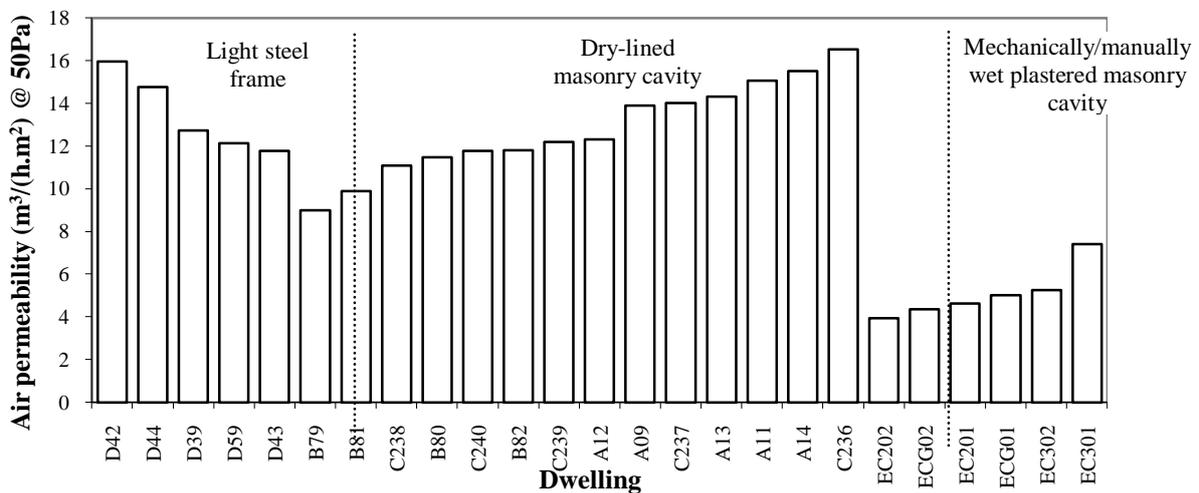
Figure 3: Mean air permeability of the tested dwellings by construction type
