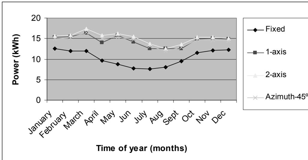
Figure 4.: PV power output for different solar tracking devices
