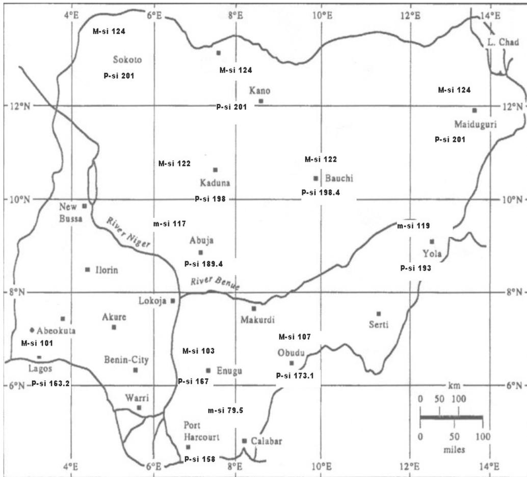
Figure6: shows energy output (Kwh/m<sup>2</sup>/annum) for various locations and types of PV cells Mono crystalline silicon (M-si) and Polycrystalline silicon (P-si).
