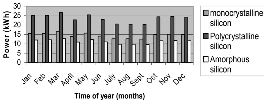
*Figure 3: Solar PV output for different PV cells*
