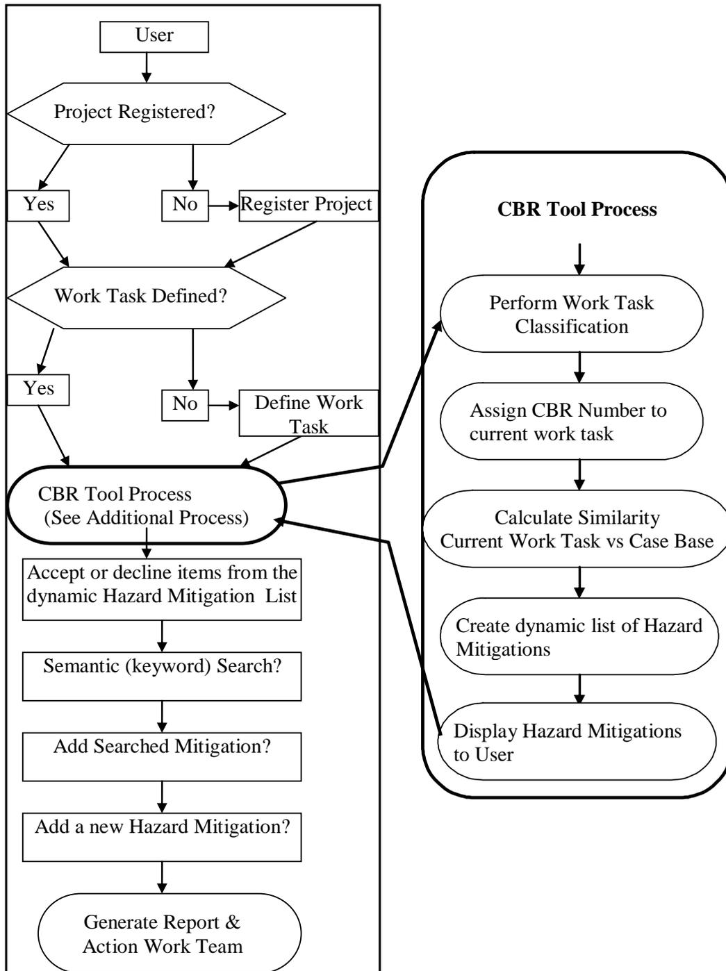
**Figure 4:** Process flow chart for CBR tool
