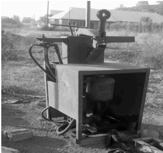
Figure 1: Nature of hydraform machine. (Source: field work, 2024)
