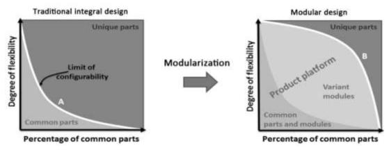
Figure 1. From integral to modular product architecture (Jensen et al. 2013)
