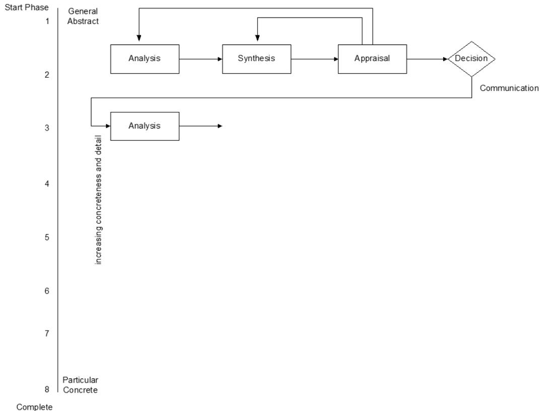
Figure 1: Model of the design process (from Markus 1972)
