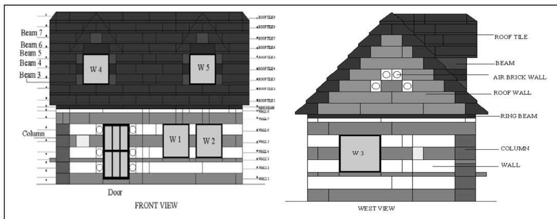
Figure 2: Elevation view of House Model
