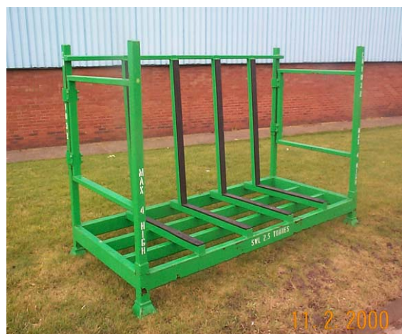
Figure 2 – LE (left) and CB (right) Stillages (reprinted with courtesy of Pilkington) Most of the larger stillages used by Pilkington can only be carried by a special truck and trailer system called a Floatliner, which is unique in the fact that it loads itself without the use of a forklift. The truck backs the trailer onto the stillage and the
