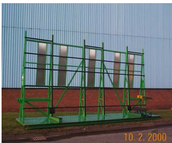
Figure 2 – LE (left) and CB (right) Stillages (reprinted with courtesy of Pilkington) Most of the larger stillages used by Pilkington can only be carried by a special truck and trailer system called a Floatliner, which is unique in the fact that it loads itself without the use of a forklift. The truck backs the trailer onto the stillage and the
