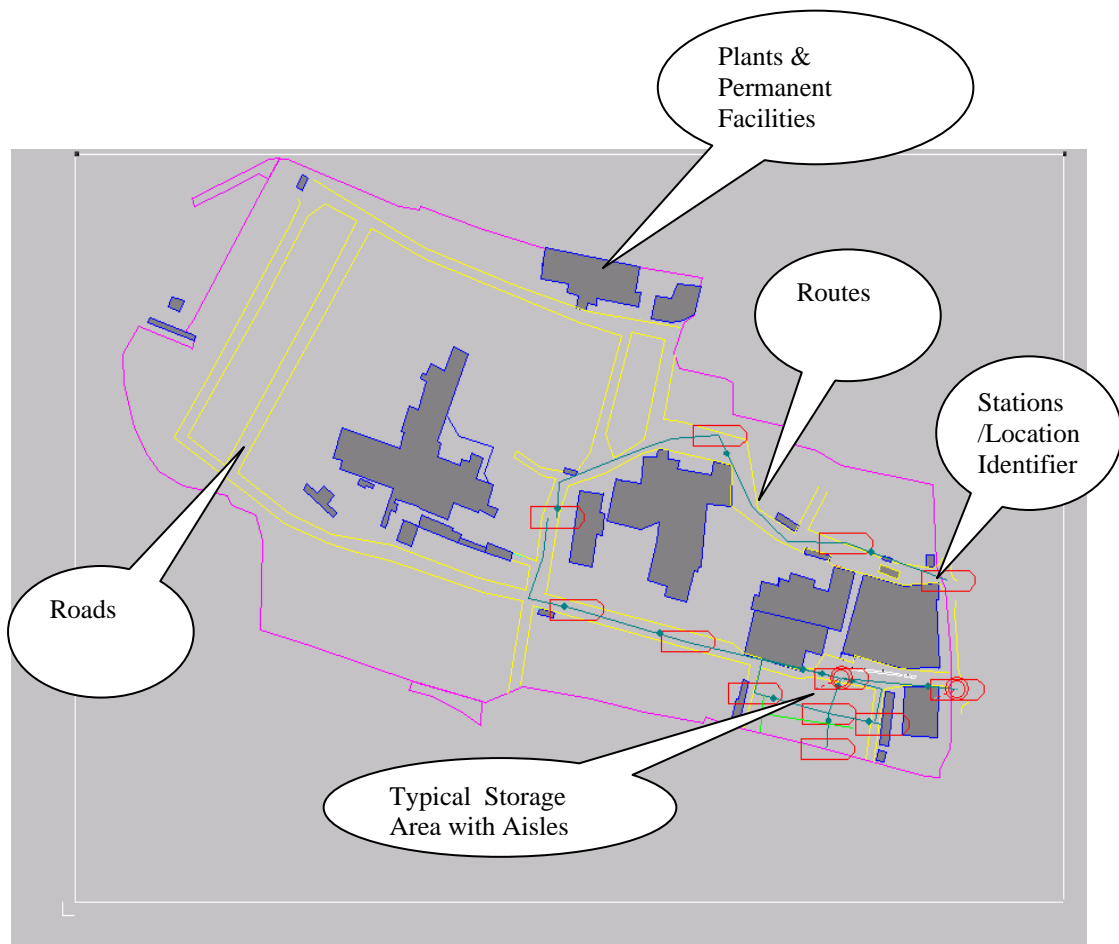
Figure 6: Sample layout and modelling of stockyard operations in ARENA
