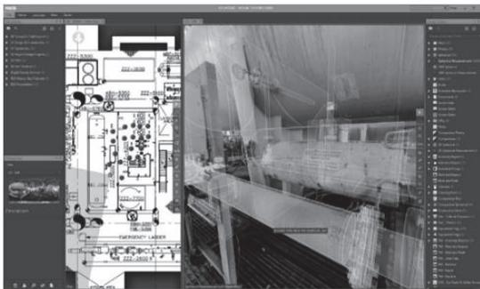
*Figure 1: VAM R2S graphical user with 360-degree photographs & databases interface*
