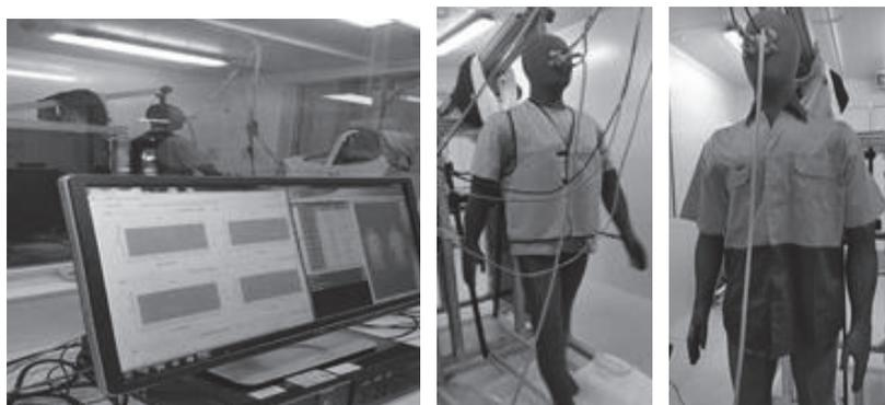
Figure 3: Manikin Tests: left: control room and cloud data; middle: 100% cotton innerwear and polyester safety vest test; right: 100% cotton shirt test
